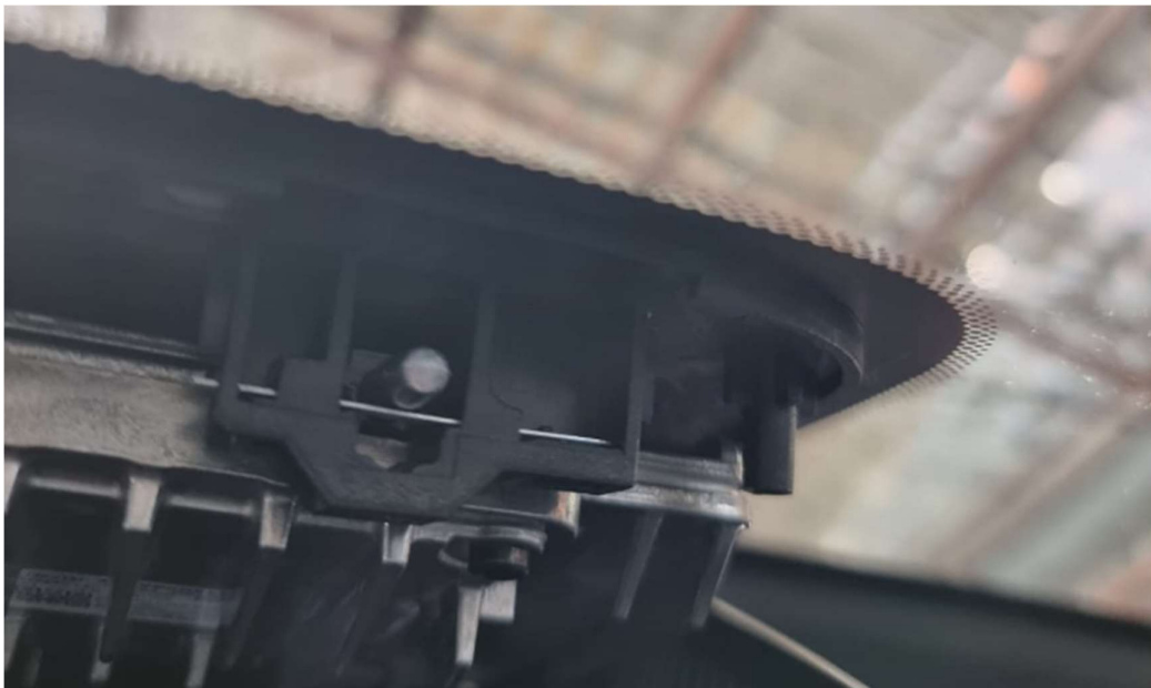
Figure 2: Incorrectly mounted, the position stud is incorrect.
